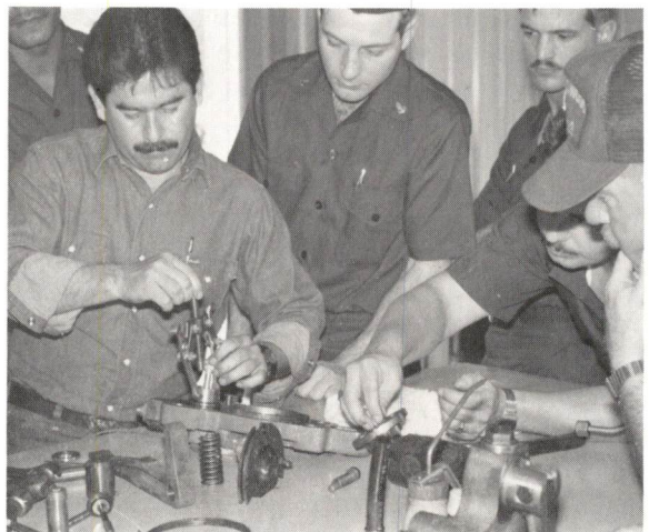
Students, under the instruction of Mr Garcia, complete tear down and rebuild of the hammer's fuel pump assembly.
