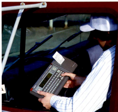
Geostar navigation system in truck cab
